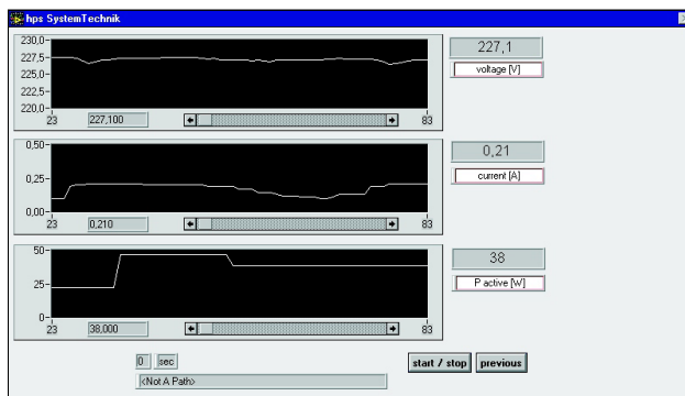
Data logger with three channels
